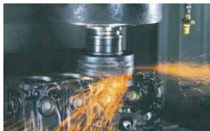
使用住友CBN刀片进行铸铁切削 Cast iron cutting by SUMIBORON inserts
