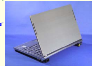
AZ91 Magnesium alloy cover for lap top computer
