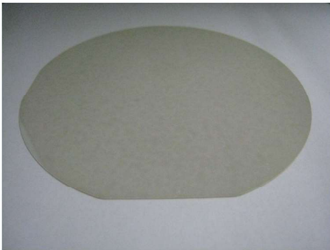
Fig. 3. Photograph of non-core 4-inch GaN substrate.
