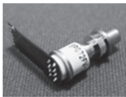
Photo 1. Burst-Mode receiver for 50G-EPON OLT
