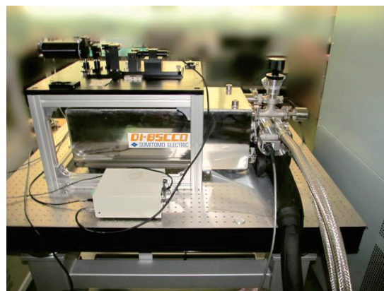
Photo 3. Magnet for hard disk inspection (Courtesy of NEOARK CORPORATION)
