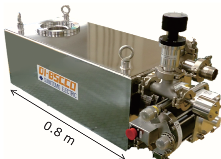
Photo 2. 20 K conduction cooled magnet
