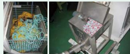
Crush and reuse of resin scraps
