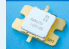
GaN HEMT Sumitomo Electric Device Innovations, Inc.
