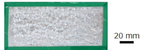
Photo 1. Appearance of a Mg alloy, which contains 139 ppm of Fe and 0.19 wt% of Al, after a 98-hour salt spray test
