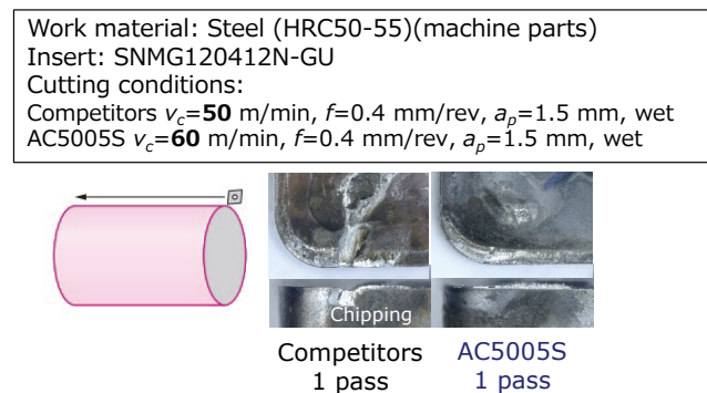
Fig. 13. Example of machining with AC5005S (4)
