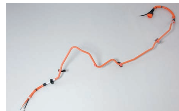
Under-floor pipe-shielded wiring harness
