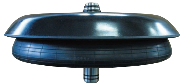
An air spring used on railway carriages
