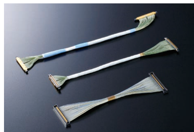
Micro coaxial cable assembly used in mobile phones
