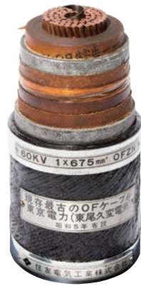
Japan's first single-core 66 kV OF 675 mm 2 cable
