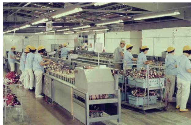
Sayama Works harness assembly line
