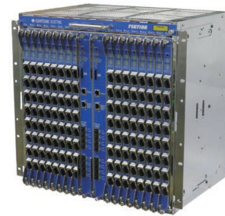
FSU7100 series, GE-PON center equipment for North American CATV operators
