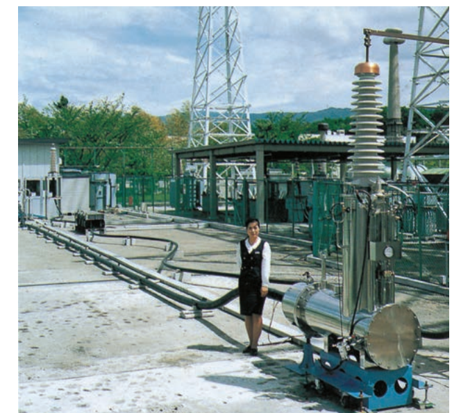
30 m high-temperature superconducting cable prototype
