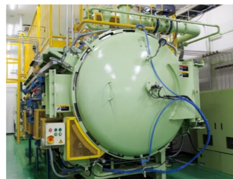
Zinc selenium (ZnSe) synthesis furnace
