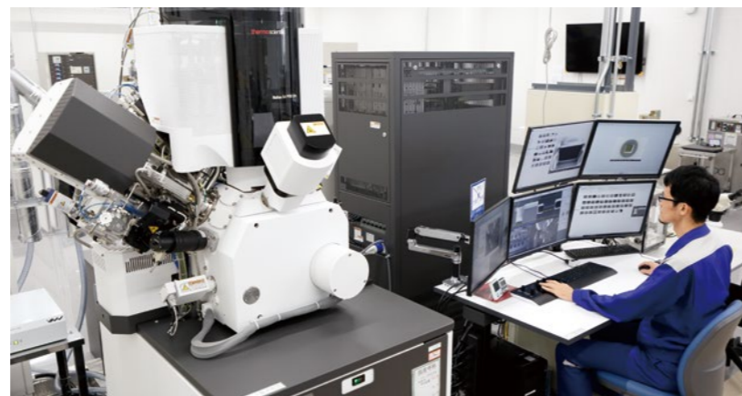
Focused Ion Beam Scanning Electron Microscope (FIB-SEM) is the main equipment for cross section preparation and observation.
