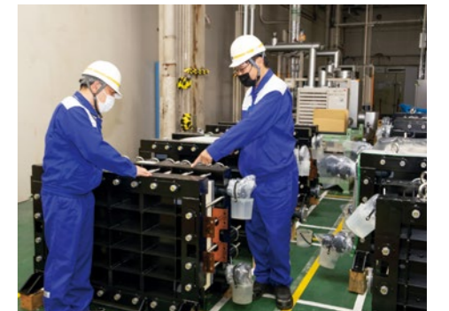
Closely check completed cell stacks
